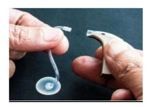
1. Detach the tube from the hearing aid with a firm tug. Be careful not to bend the tubing as a bend will stop the sound from going through to your ear from the hearing aid.
