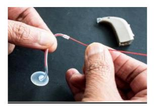
2. Insert the cleaing wire into the top of the detached tubing. Push it all the way through the tubing to clear any wax or debris.
