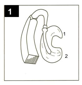
The earmould has two main parts: The 'hook' at the top (1) and the 'meatus' at the bottom (2).
