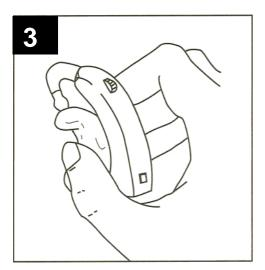
Hold the earmould between your thumb and forefinger. The 'hook' should point forwards and the meatus should point towards your ear.
